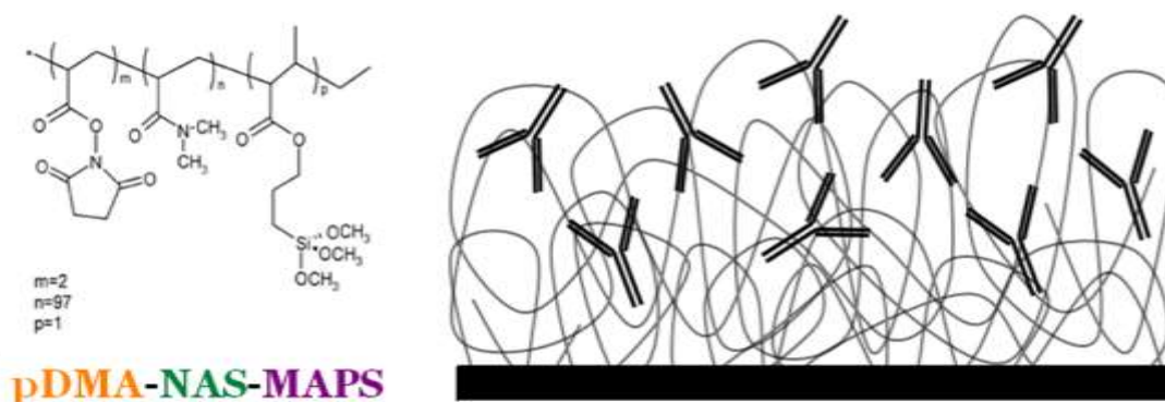
Figure 1 (a) The three major components of the polymer are DMA, NAS and MAPS in ratio 97:2:1. NAS provides the active groups, which specifically bind amine functional groups on the probe, the MAPS covalently binds to the oxide surface and DMA adsorbs to the oxide surface and provides the backbone of the polymer. (b) The polymer swells upon hydration to provide a near liquid environment for the probes. [2]
